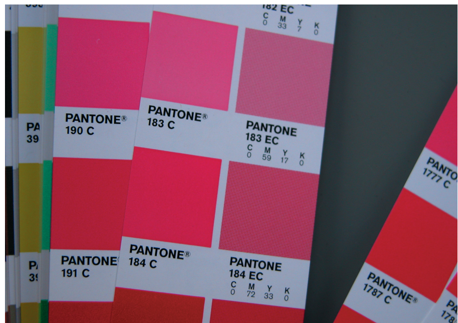
Fig. 5: The Pantone-to-process swatchbook lets you judge whether a CMYK simulation of a Pantone colour is a close enough match to satisfy your needs – and provides a 'tint formula' for achieving that simulation.
