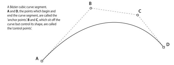
The location of these points is of course represented by their x and y co-ordinates, which are numerical values – and that is very tasty fare for a computer! To store this curve in computer memory, all we need are these four sets of co-ordinates. The curve in a sense 'does not exist', but drawing software like Illustrator can render it on the screen or on the printer whenever it is required.
