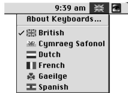
Fig. 23 The Macintosh keyboard selection menu, set up to switch between six alternate language mappings between keys pressed and characters accessed.
